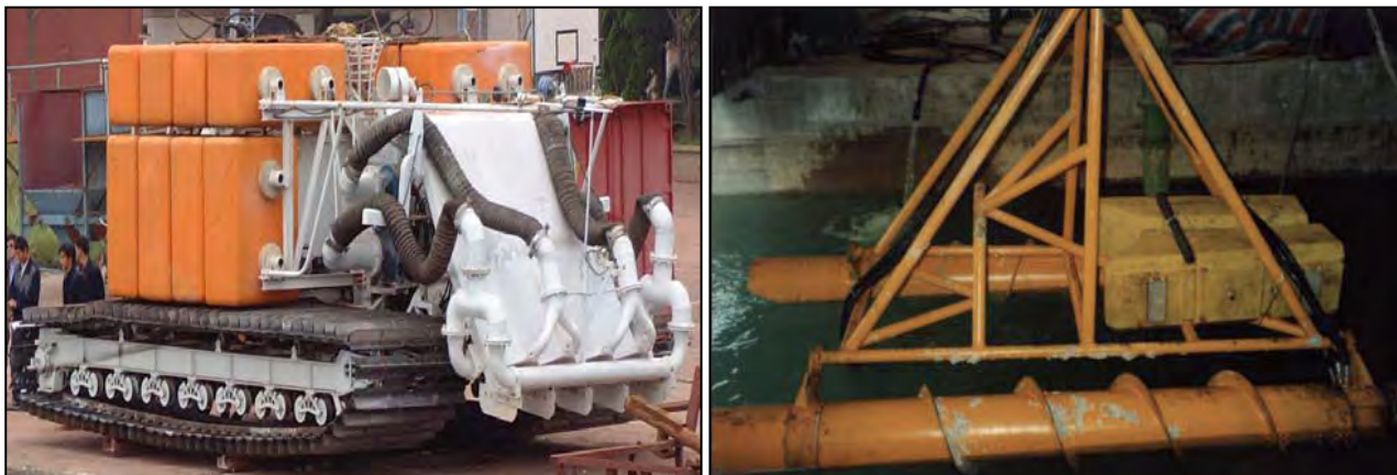
Figure 5.16 Chinese pilot scale tracked and test screw-drive subsea vehicles
