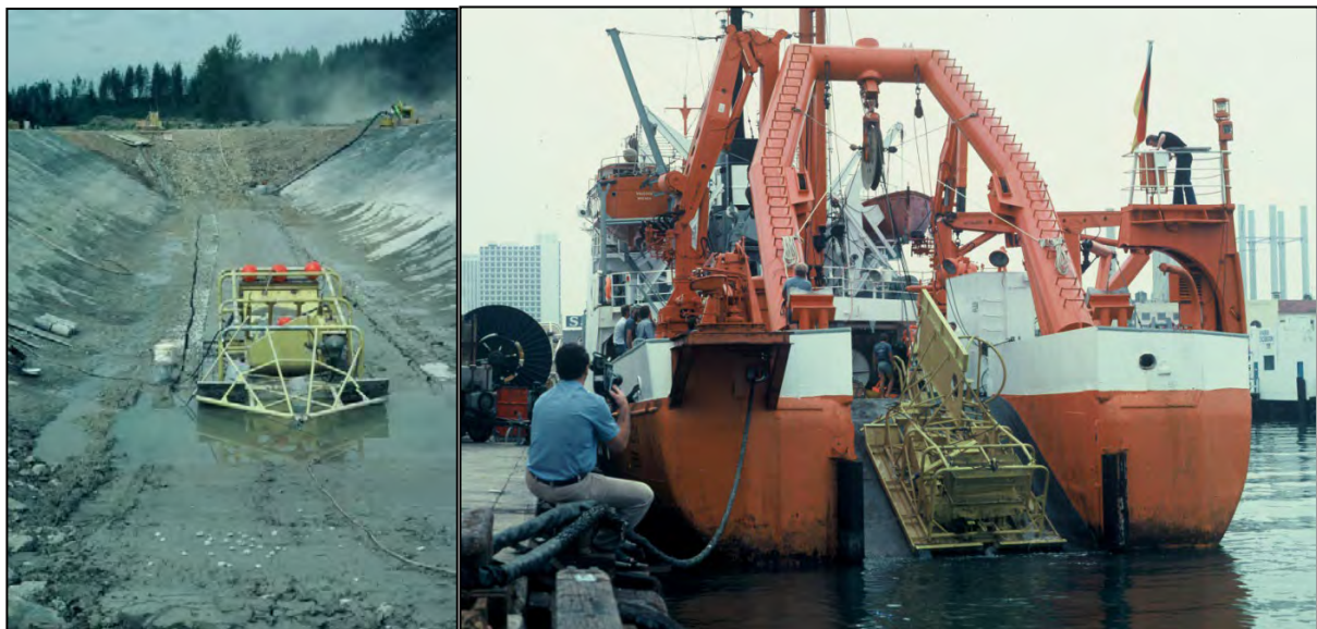
Figure 5.8 INCO electro-hydraulic collector test; DOMCO hydraulic collector launch &amp; recovery test on the RV Valdivia
