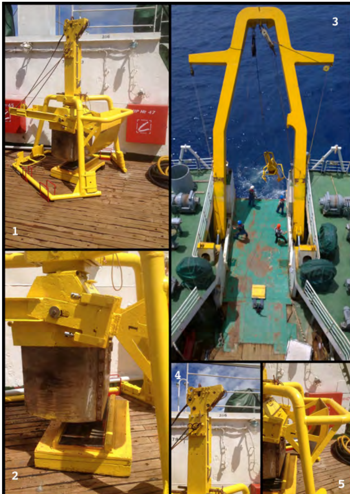
Figure 7.14 Details and recovery of the YMG box-corer
