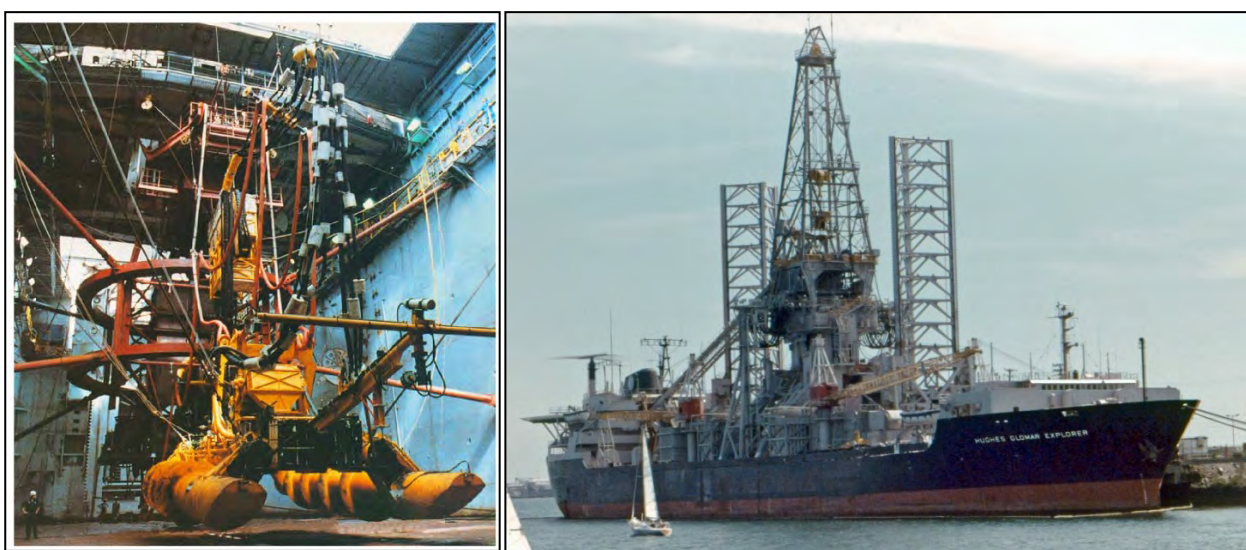
Figure 5.11 OMCO Screw-drive collector and pilot mining vessel, the USNS Hughes Glomar Explorer
